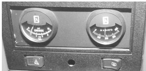
At 40 mph in 2nd gear, the ammeter reads 180A. This is the most efficient gear for this speed.
